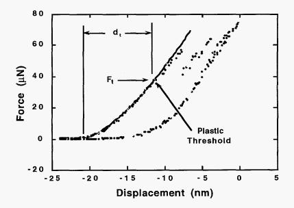
**Figure 1** A typical loading curve for a 200 nm Au film on a glass substrate. The solid line illustrates the fit of the Hertzian relationship to the data, which permits an evaluation of the quantities  $F_t$  and  $d_t$ .
