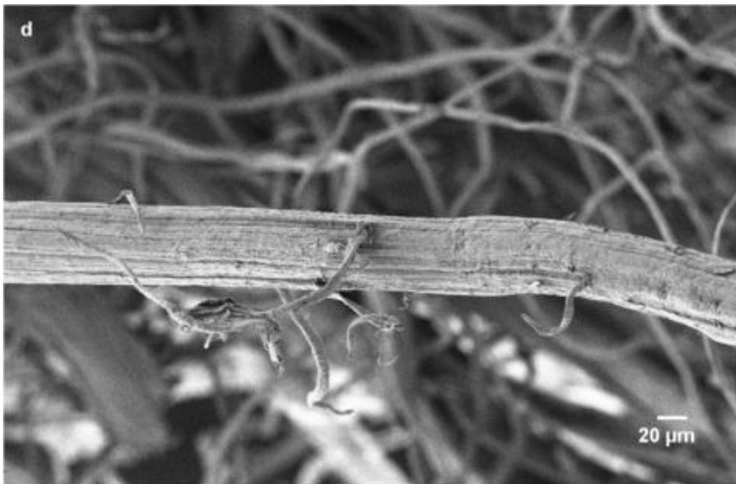
**Fig. 3d.** FESEM micrographs of *Agave* leaves and fibres: (a) longitudinal section, (b) cross section of the arch (Murherjee and Satyanarayana,1984), (c) raw, (d) alkali-treated, and (e) bleached
