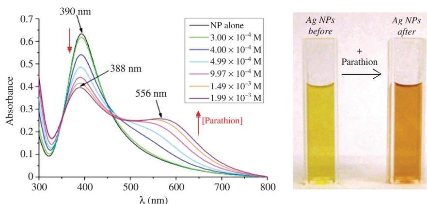
**Fig. 2** Changes in the colloid SPR absorbance band and colloid color of Ag NPs upon the interaction with parathion. The red arrows indicate the direction of the SPR peak with increasing parathion concentration.
