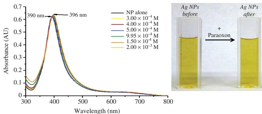
**Fig. 3** Changes in the colloid SPR absorbance band and colloid color of Ag NPs upon titration with paraoxon-ethyl.
