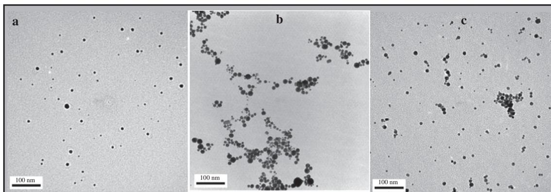
**Fig. 4** TEM images of (a) Ag NPs, (b) Ag NPs in the presence of parathion and (c) Ag NPs in the presence of paraoxon-ethyl. The scale bar represents 100 nm.
