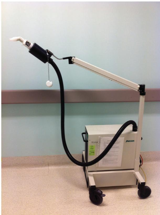
**Figure 1** Picture of an EcoScreen® collection device.
