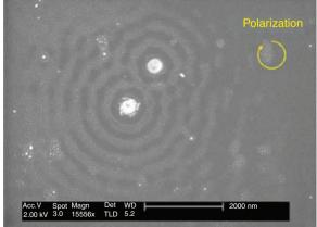
**Figure 11:** SEM image of the silicon surface after laser irradiation. The circularly polarized femtosecond laser at 400 nm was irradiated at 0.08 J/cm<sup>2</sup>. The two white circles are the 200-nm-diameter gold spheres. The interference period is 400 nm approximately [55].
