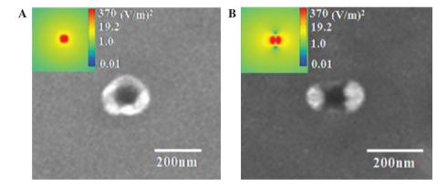
**Figure 5:** SEM images of the fabricated nanohole with 200-nm gold sphere on silicon substrate. The pulse duration is 150 fs, laser fluence is 0.2 J/cm<sup>2</sup>, and the hole is ablated by a single shot irradiation. (A) and (B) show the hole obtained with circular polarization and linear polarization, respectively. The inset shows the optical field intensity distribution inside the Si substrate (*z*=-1.25 nm) [27].
