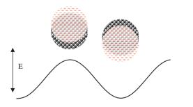
**Figure 1:** A schematic representation of the interaction of a small metal particle with EM field. Assuming that the heavy ion system is static, the electrons oscillate following the incident *E* field.
