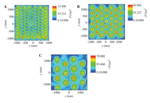
**Figure 8:** Calculated optical near-field intensity  $(|E/E_0|^2)$  distribution on a gold substrate surface when gold nanospheres with diameter of 200 nm are arrayed hexagonally and irradiated by optical wave at a wavelength of 800 nm. The field distribution is shown for three intersphere distances: (A) 200 nm (touching spheres), (B) 400 nm, and (C) 785 nm. The white circle represents the sphere delineation in (A) [43].
