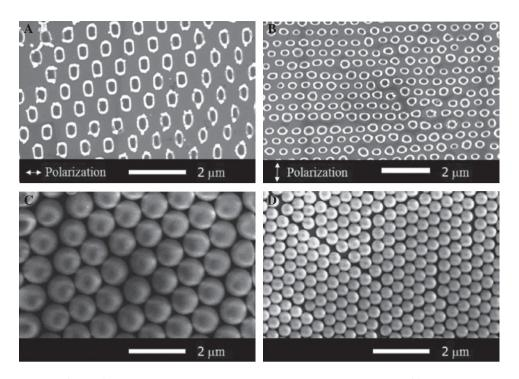
**Figure 9:** (A and B) SEM images of the Si surface after femtosecond laser irradiation. (A) 800 nm with fluence of 288 mJ/cm<sup>2</sup>; (B) 400 nm with fluence of 57 mJ/cm<sup>2</sup>. (C and D) SEM images of ordered monolayer PS spheres in hexagonal array on silicon substrate. (C) The diameter is 800 nm. (D) The diameter is 450 nm [48].
