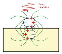
Figure 3: Conceptual illustration of EM coupling between a metallic sphere and a substrate.
