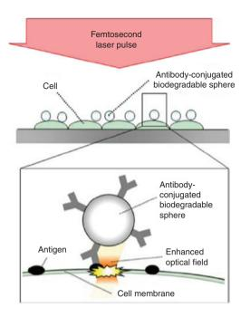
**Figure 13:** Conceptual diagram of biodegradable sphere-mediated perforation of a cell membrane using a femtosecond laser. The sphere works as a microlens, and a femtosecond laser irradiation generates a strongly enhanced optical field under the sphere to perforate the membrane [71].
