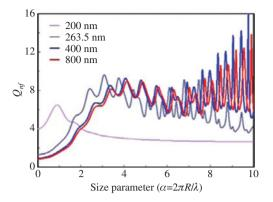
**Figure 6:** Dependence of the near-field efficiency on the size parameter for four wavelengths [34]. The near-field efficiency  $Q_{nf}$  is starting from  $\alpha = 0.01$ .
