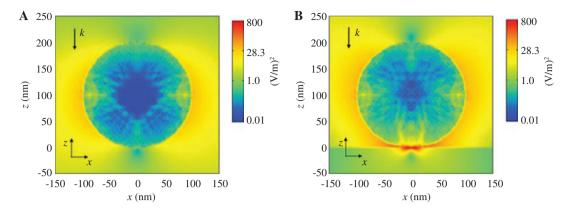
**Figure 4:** Optical field intensity ( $|E/E_0|^2$ ) distribution for a 200-nm gold sphere (A) in vacuum and (B) on silicon substrate. The 800-nm incident wave polarization is linear and the *E* vector is parallel to the *x* axis [27].
