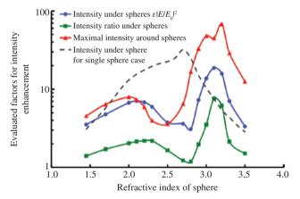
**Figure 10:** Evaluated factors for intensity enhancement when the hexagonally close-packed sphere array with the diameter of 200 nm is placed on an Si substrate, as a function of the sphere's refractive index ( $\lambda$ =400 nm) [51].
