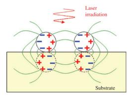
**Figure 7:** Conceptual illustration of EM coupling between metallic spheres and a substrate.
