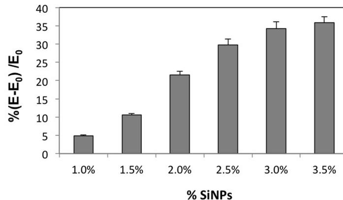
**Fig 2. Compressive modulus of pAAm hydrogel nanocomposites.** Percent relative compressive moduli of pAAm hydrogels as a function of 4 nm silica nanoparticle concentration. The values for relative compressive modulus were calculated by normalizing the values for pAAm-SiNP nanocomposite gels ( $E$ ) to those for neat pAAm gels ( $E_0$ ). Error bars indicate the standard deviation of triplicate measurements.
