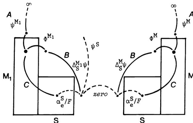
Fig. 1. Sketch to put in evidence the components of the electrode potential. Work along path B is expressed by eqn.(10) in the text. Work from  $M(M_1)$  to infinity (path A) and work from  $M(M_1)$  to S (path C) define the two other conceptually possible single electrode potentials.
