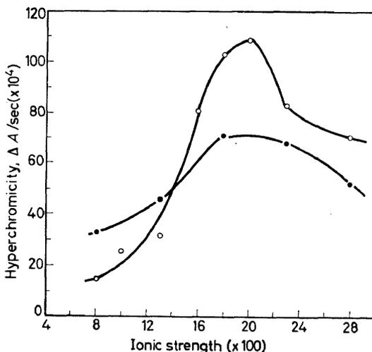
Figure 4. The initial rate of development of hyperchromicity of yeast RNA treated with ribonuclease as a function of ionic strength of the medium; all determinations in H<sub>2</sub>O-acetate buffer, pH 5.0, with appropriate amounts of added sodium chloride
