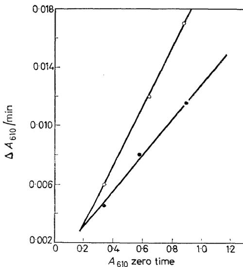
Figure 3. The concentration dependence of the proteolytic hydrolysis of ordinary (●) and deutero (○) phycocyanin; the rate of decrease of absorbancy in the presence of  $\alpha$ -chymotrypsin is plotted against protein concentration; enzyme concentration, 0.067 mg/ml; 0.01 M phosphate buffer, H<sub>2</sub>O, pH 7.23
