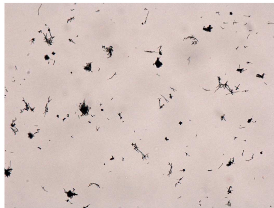
Figure 6. Low-magnification light micrograph of a filter used for counting aerosolized carbon nanofibers (CNFs). Note that some of the CNFs are agglomerated.
