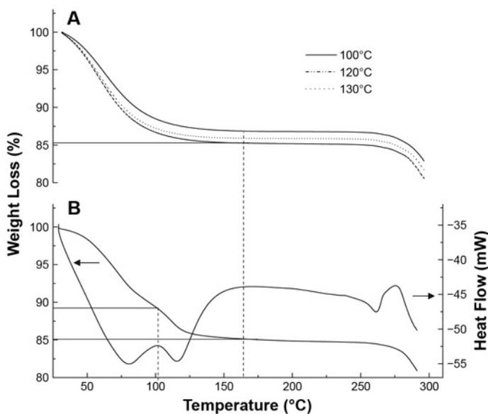
**Figure 7.** Thermogravimetric thermograms of supercritical assisted atomization-processed cromolyn sodium at different temperatures (a); thermogravimetric and differential scanning calorimetry traces of untreated cromolyn sodium (b). All samples have been analyzed after 12 months of storage.
