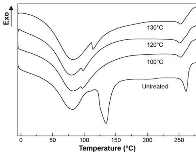
**Figure 6.** Differential scanning calorimetry thermograms of untreated and supercritical assisted atomization-processed cromolyn sodium at different temperatures after 12 months of storage. Exo indicates exothermic flow.
