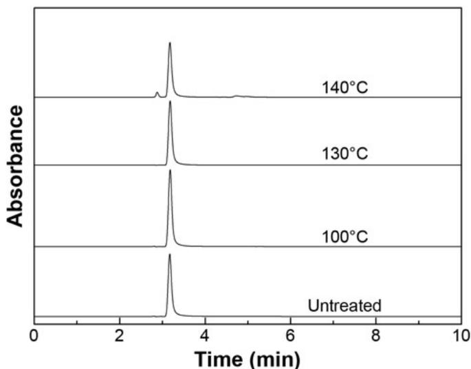
**Figure 4.** High-performance liquid chromatography trace of unprocessed and supercritical assisted atomization micronized cromolyn sodium at 50 mg/mL at different temperatures.
