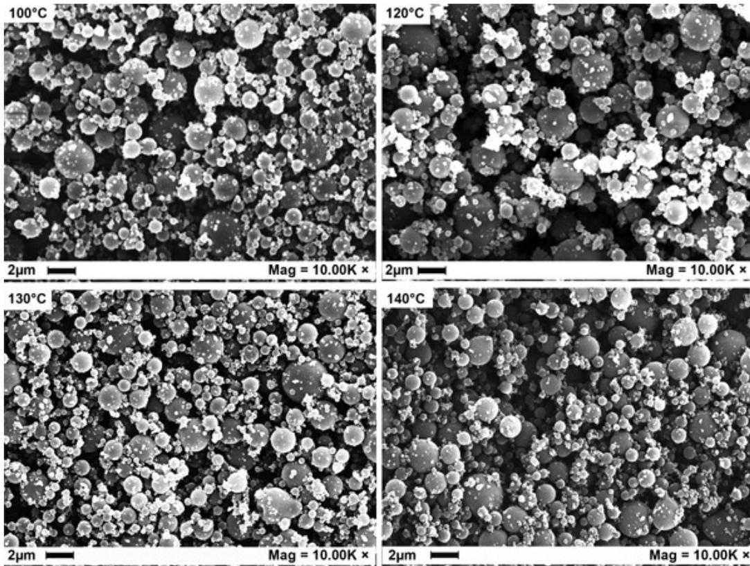
**Figure 1.** Scanning electron microscopy photomicrographs of cromolyn sodium precipitated by supercritical assisted atomization at 50 mg/mL at various precipitation temperatures.
