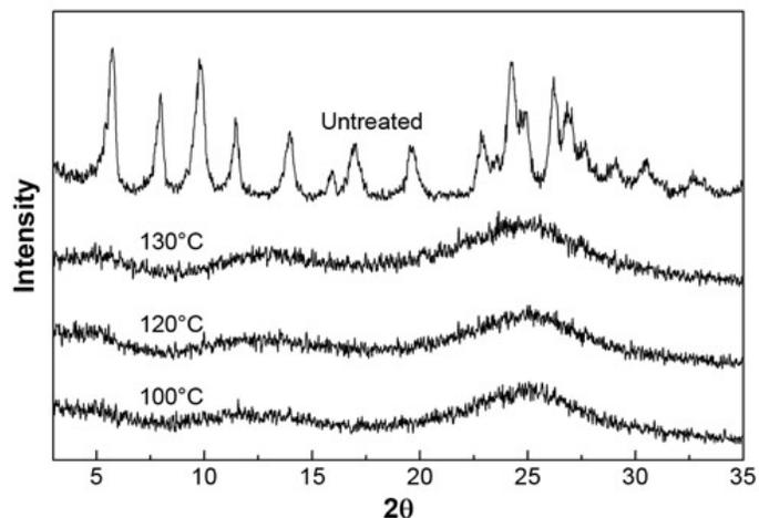
**Figure 5.** X-ray powder diffraction patterns for untreated and supercritical assisted atomization-processed cromolyn sodium at different temperatures.
