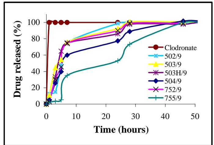
Figure 4. In vitro release profile of clodronate from microspheres produced with poly(D,L-lactide-co-glycolide) copolymers ( $n = 3$ ,  $SD < 5\%$ ).
