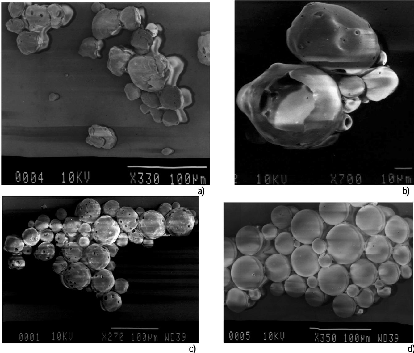
Figure 1. Photomicrographs of RG 503 microparticles. Obtained with: A, 1:5 inner water/oil emulsion volume ratio; B, temperature-raising rate  $10^\circ\text{C}/\text{min}$ ; C, 1:16 inner water/oil emulsion volume ratio and temperature-raising rate  $1^\circ\text{C}/\text{min}$ ; and D, 1:16 inner water/oil emulsion volume ratio, temperature-raising rate  $1^\circ\text{C}/\text{min}$  and NaCl 2% wt/vol in the external aqueous phase.
