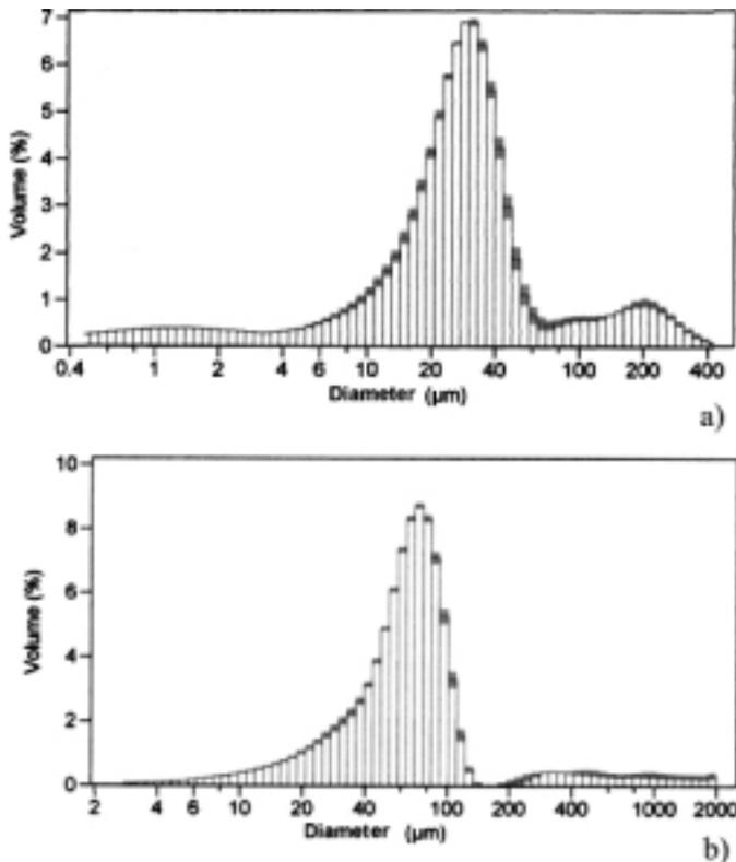
Figure 2. Particle-size distribution of batches. A, 502/9 ( $d_{50\%}$  26.85  $\mu\text{m}$ ,  $d_{90\%}$  93.58  $\mu\text{m}$ ). B, 504/9 ( $d_{50\%}$  64.42  $\mu\text{m}$ ,  $d_{90\%}$  113.1  $\mu\text{m}$ ).
