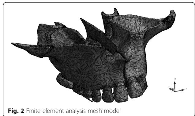
**Fig. 2** Finite element analysis mesh model
