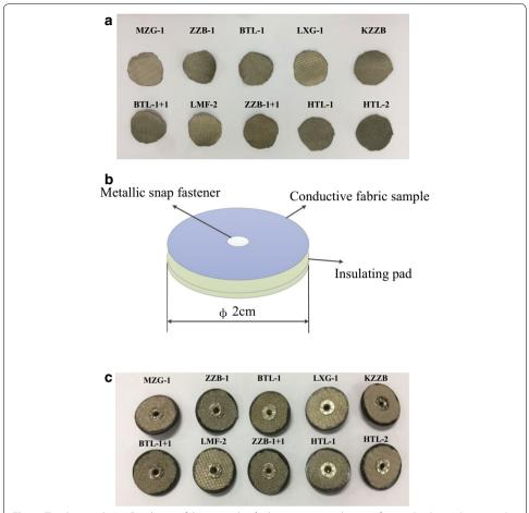
$\textbf{Fig. 1} \ \ \text{Textile samples.} \ \textbf{a} \ \ \text{Conductive fabric samples,} \ \textbf{b} \ \ \text{decomposition diagram for textile electrodes,} \ \textbf{c} \ \ \text{textile electrodes}$
