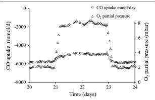
**Fig. 2** CO consumption profile of a continuously operating *C. autoethanogenum* gaseous fermentation undergoing varying levels of oxygen addition. At 2 mbar oxygen concentration CO uptake is stable at approximately 5900 mmol/day which, when oxygen is increased to 8 mbar, reaches a reversible equilibrium of CO uptake around 5000 mmol/day
