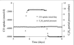
**Fig. 1** CO consumption profile of a continuously operating *C. autoethanogenum* gaseous fermentation undergoing addition of ethylene by sparging with ethylene containing Nitrogen. CO consumption remains stable around 5800 mmol CO/day
