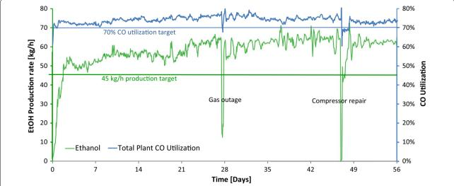
Fig. 3 Ethanol production and carbon monoxide utilization profiles over an 8 week period. Data collected at the Beijing Shougang LanzaTech New Energy Science & Technology Co., Ltd, a 0.1 Mgy ethanol capacity demonstration facility
