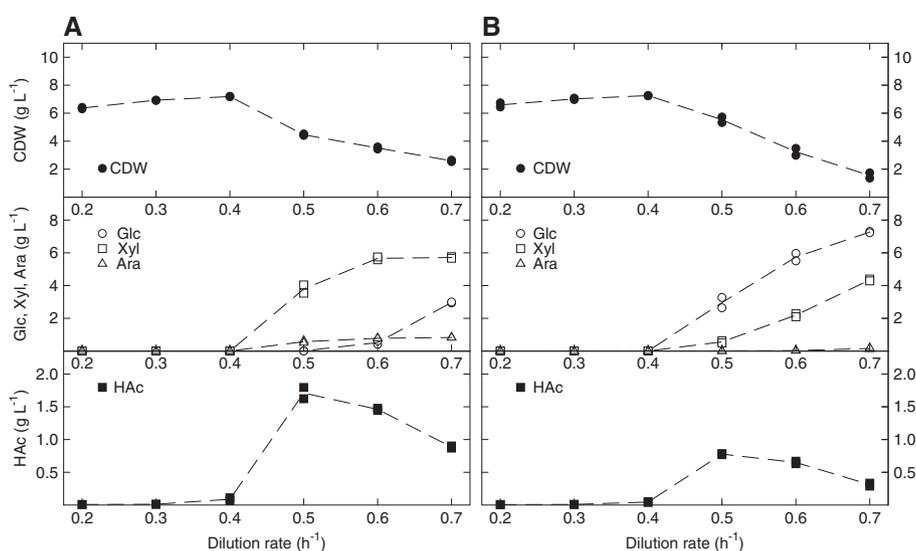
**Figure 2 Growth of *E. coli* AF1000 (A) and PPA652ara (B) on glucose, xylose and arabinose in continuous mode without product formation.** Parameters: cell dry weight (CDW, filled circles), glucose (Glc, open circles), xylose (Xyl, open squares), arabinose (Ara, open triangles) and acetic acid (HAc, filled squares). Each dilution rate was tested in duplicate and the mean values of the two sample series are represented as dashed lines.
