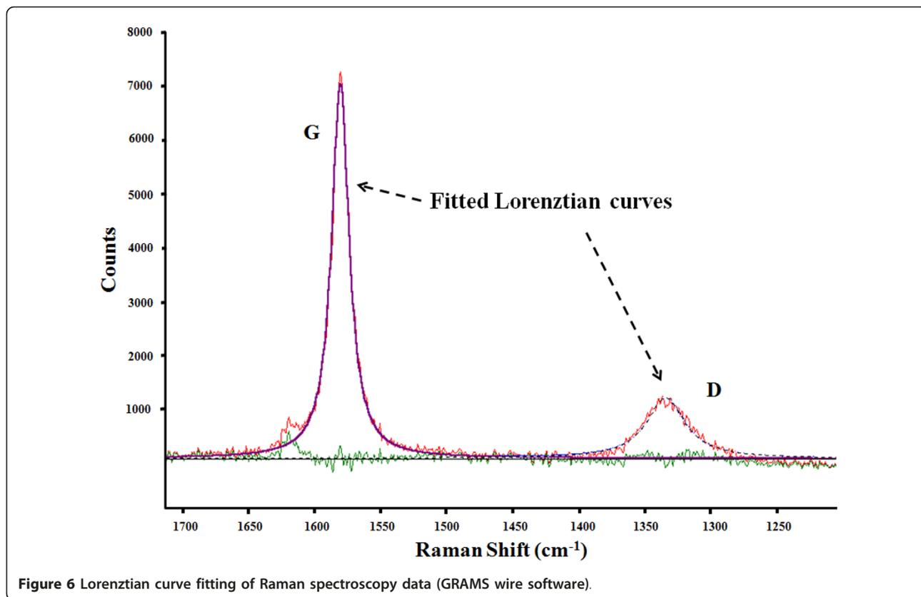
Figure 6 Lorentzian curve fitting of Raman spectroscopy data (GRAMS wire software).
