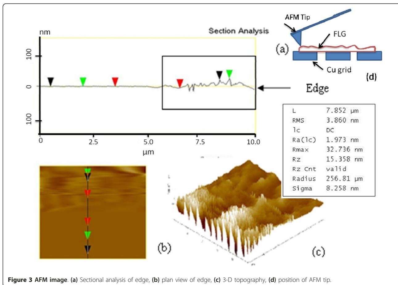
**Figure 3 AFM image.** (a) Sectional analysis of edge, (b) plan view of edge, (c) 3-D topography, (d) position of AFM tip.
