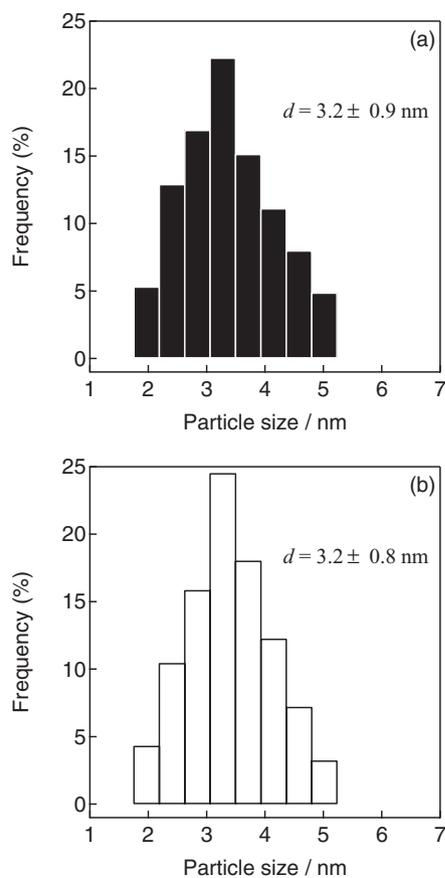
Figure 3. Pt particle size distribution for (a) Pt/C and (b) RuO<sub>2</sub>ns(0.3)-Pt/C.
