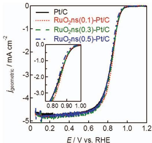
Figure 5. Linear sweep voltammograms of RuO<sub>2</sub>ns(*n*)-Pt/C, with *n* = 0, 0.1, 0.3 and 0.5 at  $\omega = 1600$  rpm,  $v = 10$  mV s<sup>-1</sup> in 0.5 M H<sub>2</sub>SO<sub>4</sub>(60°C).
