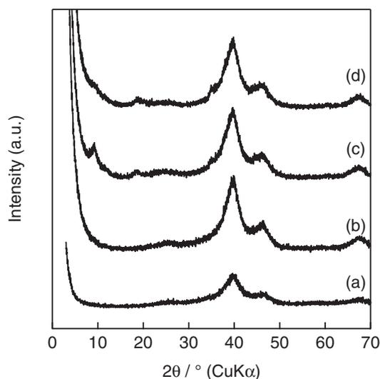
**Figure 1.** The XRD patterns of (a) Pt/C, (b) RuO<sub>2</sub>ns(0.05)-Pt/C, (c) RuO<sub>2</sub>ns(0.3)-Pt/C and (d) RuO<sub>2</sub>ns(0.5)-Pt/C.
