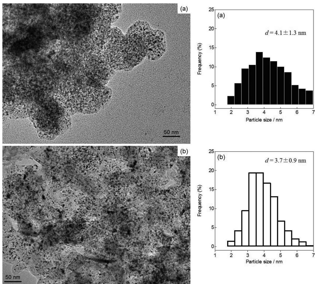
**Figure 9.** TEM images and Pt particle size distribution (a) Pt/C and (b) RuO<sub>2</sub>ns(0.3)-Pt/C composite catalyst after accelerated durability test.
