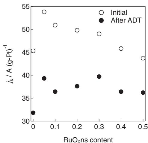
**Figure 7.** Mass activity before and after accelerated durability test as a function of the RuO<sub>2</sub>ns content.
