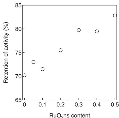
**Figure 8.** Retention of activity after accelerated durability test as a function of the RuO<sub>2</sub>ns content.
