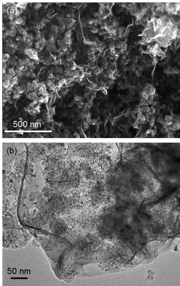
**Figure 2.** A typical (a) SEM image and (b) TEM image of RuO<sub>2</sub>ns(0.3)-Pt/C.
