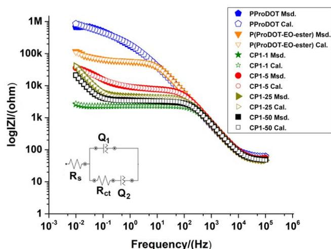
**Figure 12.** Measured and calculated impedance values of the Bode magnitude diagrams of PProDOT, P(ProDOT-EO-ester), CP1-1, CP1-5, CP1-25 and CP1-50. The inset shows proposed equivalent circuit model (ECM) adopted for all polymer samples.
