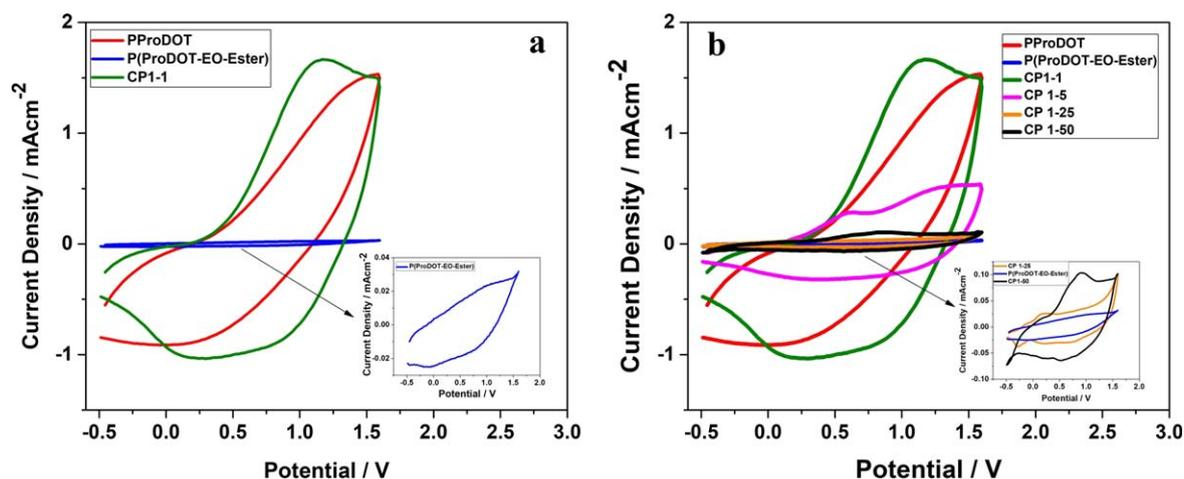
**Figure 4.** The CVs of (a) the PProDOT, P(ProDOT-EO-Ester), and CP1-1, inset in Fig. 4a shows the CV of P(ProDOT-EO-Ester) homopolymer, (b) all homopolymers and its copolymers (PProDOT, P(ProDOT-EO-Ester), CP1-1, CP1-5, CP1-25, and CP1-50) coated on the Si/Graphene electrode at the scan rate of  $50$   $\text{mVs}^{-1}$  in  $0.1$  M  $\text{Et}_4\text{NBF}_4/\text{ACN}:\text{DCM}$  (3:1), and inset of Fig. 4b shows P(ProDOT-EO-Ester) homopolymer and copolymers of CP1-25 and CP1-50.
