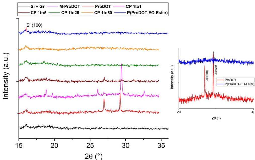
**Figure 8.** X-ray diffraction (XRD) patterns of PProDOT, P(ProDOT-EO-ester) and its copolymers. The inset figure shows that the particular ProDOT peaks are indexed in comparison to its ester derivative.
