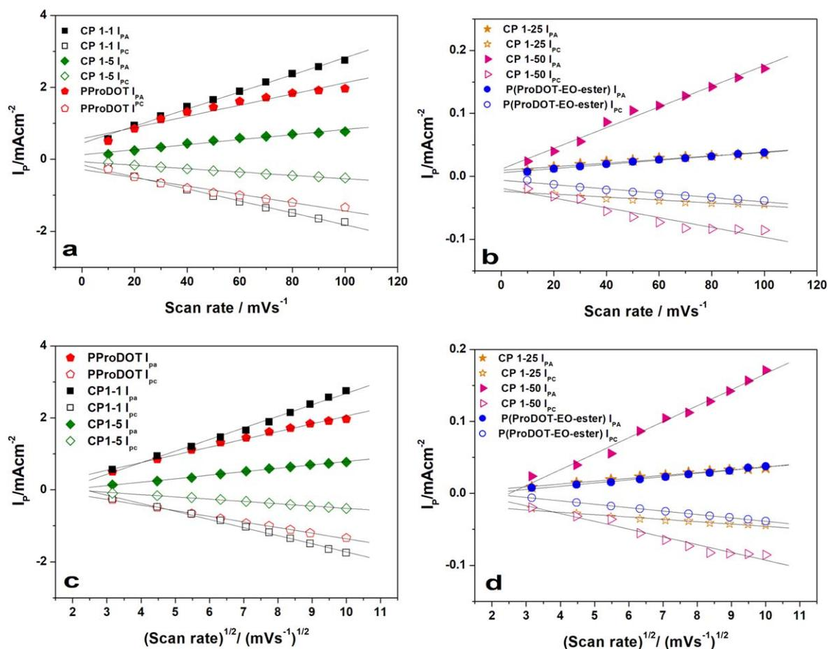
**Figure 5.** Scan rate vs current density and (a) and (b), square root of the scan rate vs current density plots (c) and (d) for PProDOT, P(ProDOT-EO-ester), CP1-1, CP1-5, CP1-25, and CP1-50.
