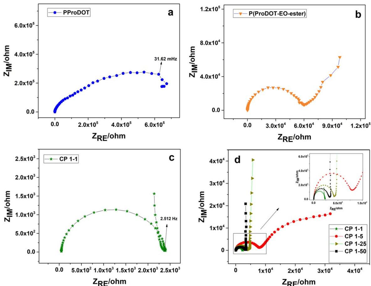
**Figure 11.** Nyquist diagrams for (a) PProDOT (b) P(ProDOT-EO-ester), (c) CP1-1, and (d) CP1-1, CP1-5, CP1-25 and CP1-50 for comparison. Frequency range: 10 mHz–100 kHz, 10 mV DC amplitude at open circuit potential conditions.
