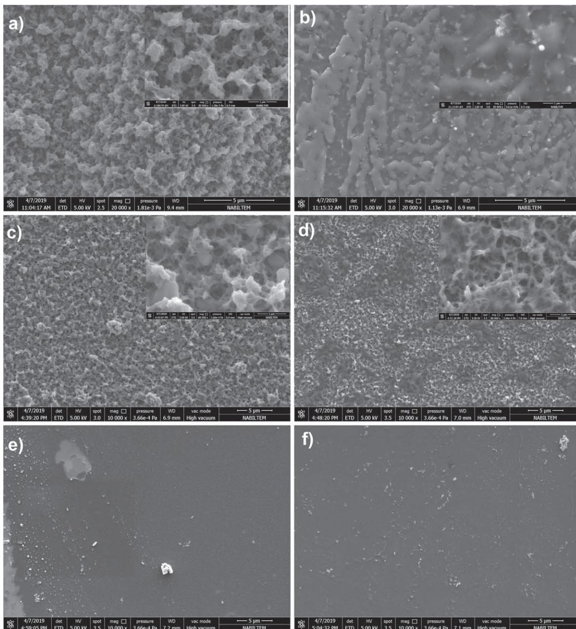
**Figure 9.** FEGSEM images of (a) PProDOT, (b) P(ProDOT-EO-ester), (c) CP1-1, (d) CP1-5, (e) CP1-25, and (f) CP1-50, each scale bar is 5  $\mu\text{m}$ . The insets show high magnification images of the corresponding films, and inset scale bar is 1  $\mu\text{m}$ .
