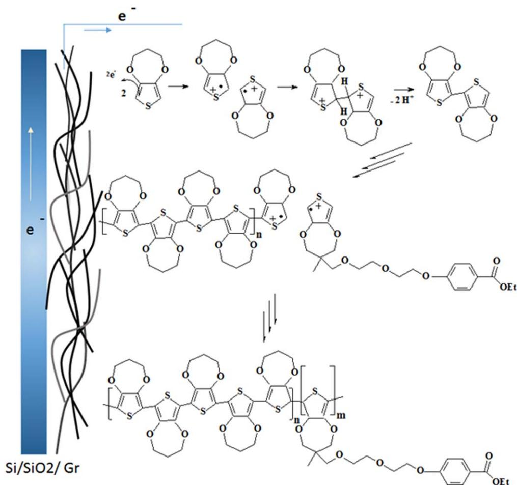
**Figure 1.** Schematics of electrochemical deposition and growth of copolymer on Si/graphene.
