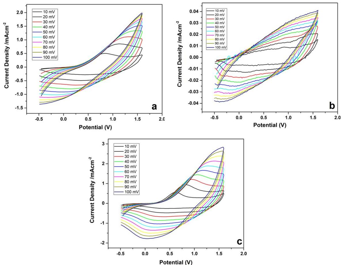
**Figure 3.** Cyclic voltammetry of (a) PProDOT, (b) P(ProDOT-EO-ester), (c)  $[\text{ProDOT}]_0/[\text{ProDOT-EO-ester}]_0 = 1:1$ , in monomer-free solution, in the potential range:  $-0.5$ – $1.6$  V, in  $0.1$  M  $\text{Et}_4\text{NBF}_4/\text{ACN}:\text{DCM}$  (3:1) at scan rates between  $10$  and  $100$   $\text{mVs}^{-1}$ .
