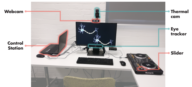
Figure 2: Experimental setup used during the study. It consists of a thermal camera, web-camera, eye-tracker and a slider.
