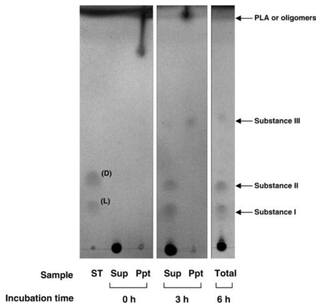
FIG. 3. Thin-layer chromatogram of the degradation products from PLA of 220 kDa by the purified rPLD preparation. Enzyme reaction and detection of the degradation products were carried out as described in Materials and Methods. ST: mixture of authentic lactic acid (L) and lactic acid dimer (D). The black spot at the origin of each supernatant sample on the plate and 6-h incubation sample was Trisma base in the incubation mixtures.
