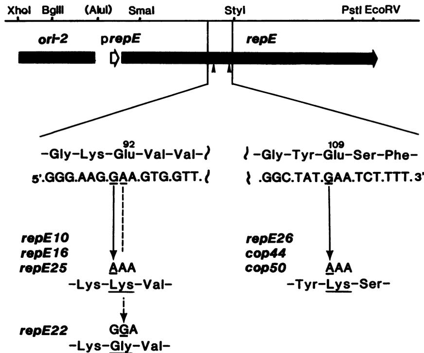
FIG. 3. Alterations of nucleotide and predicted amino acid sequences in the mini-F *repE* mutants. Amino acid numbers are based on the finding that the N-terminal methionine is processed and is not found in the mature RepE protein (29).
