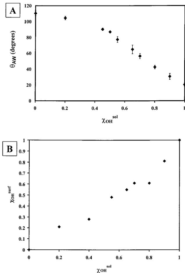
FIG. 1. Surface chemical properties of mixed SAMs. (A)  $\theta_{AW}$  of mixed SAMs formed from OH-thiol and  $\text{CH}_3$ -thiol. The data are averages for three test areas. The error bars indicate one standard deviation. (B)  $\chi_{OH}^{surf}$  in mixed SAMs as a function of the  $\chi_{OH}^{sol}$  used to form the mixed SAMs.
