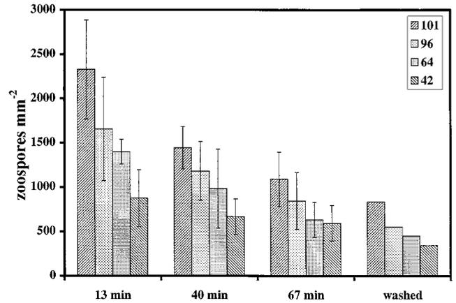
FIG. 6. Distribution of spores on patterned SAMs with  $\theta_{AW}$  of  $101^\circ$ ,  $96^\circ$ ,  $64^\circ$ , and  $42^\circ$ . The counts represent both cells that settled on the surface and swimming cells in the same focal plane. The washed counts represent settled cells only, which were recorded on video after the 70-min sample was washed.
