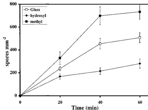
FIG. 2. Time course for zoospore adhesion to glass ( $\theta_{AW}$ ,  $\sim 40^\circ$ ), a  $\text{CH}_3$ -terminated (methyl) SAM ( $\theta_{AW}$ ,  $116^\circ$ ), and a OH-terminated (hydroxyl) SAM ( $\theta_{AW}$ ,  $<15^\circ$ ). Each point is a mean based on 30 counts; the bars indicate 95% confidence limits.
