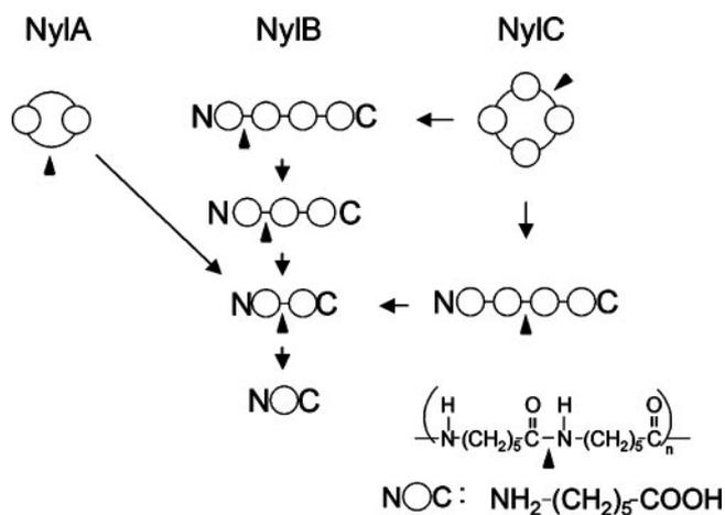
FIG. 1. Mode of degradation of nylon oligomers by the Ahx cyclic-dimer hydrolase (NylA), the Ahx dimer hydrolase (NylB), and the Ahx endo-type-oligomer hydrolase (NylC).
