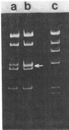
FIG. 1. Agarose gel electrophoresis of *Hind*III restriction of (a)  $\lambda$  Sam7 lysogen DNA and (b) the same DNA containing the 4.3-kb fragment (arrow) specifying tetracycline resistance from plasmid RA1. (c)  $\lambda$  DNA *Hind*III digest standard (New England Biolabs), from top to bottom: 23, 9.8, 6.6, 4.5, 2.5, and 2.2 kb.
