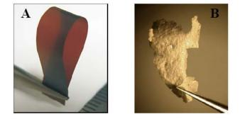
Fig. 3. Graphene derivatives. (A) Graphene-oxide laminate is tough, flexible, transparent and insulating (6). (B) Paper made in the same way as A but starting from graphene suspension (5) is porous, fragile, opaque and metallic (courtesy of R. Nair, Manchester).
