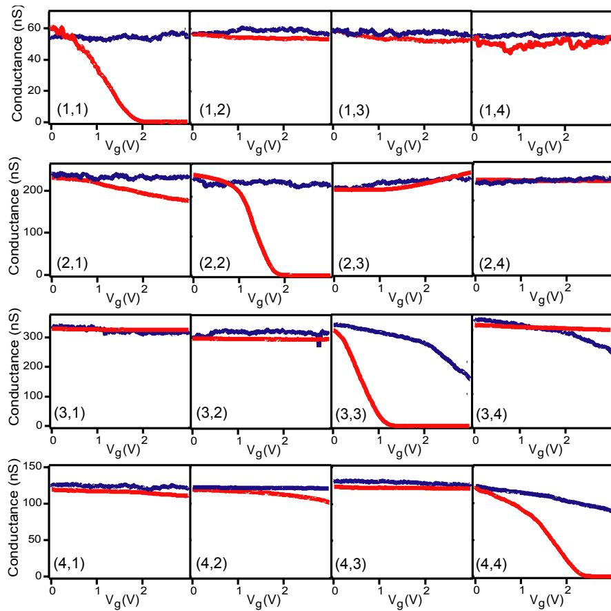
**Fig. S1.** Conductance vs. gate voltage for each cross point in the 4x4 cNW-FET array shown in Fig. 3D; The blue and red curves correspond to data recorded before and after chemical modification, respectively. Each plot corresponds to one cNW junction ( $n, m$ ). The four diagonal junctions, (1,1), (2,2), (3,3), and (4,4), were modified in this array.
