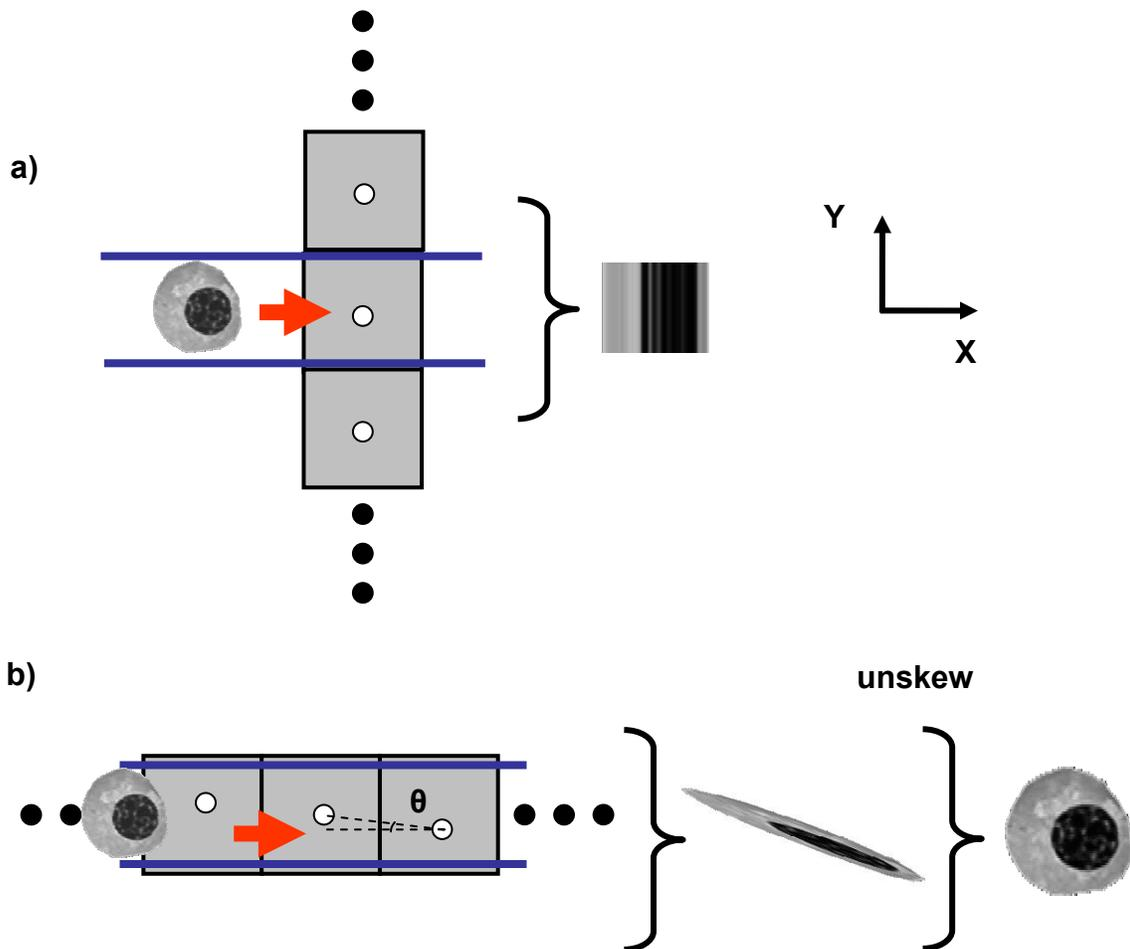
**Figure 1:** **a.** A non-OFM imaging scheme yields an image with poor quality because of the sparse sampling in the Y direction. **b.** OFM imaging scheme can achieve dense sampling in the Y direction by choosing a proper tilt angle  $\theta$ .
