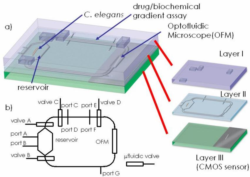
**Figure 7:** A closed-loop microfluidic lab-on-a-chip system that can incubate and perform automated imaging of a single nematode for life-cycle studies.
