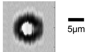
**Figure 6:** A OFM image of a 4.5 μm polystyrene microsphere.
