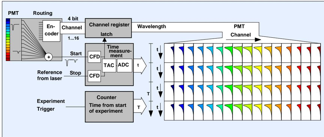
Fig. 4: Sequential recording
