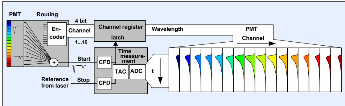
Fig. 2: Multi-wavelength TCSPC
