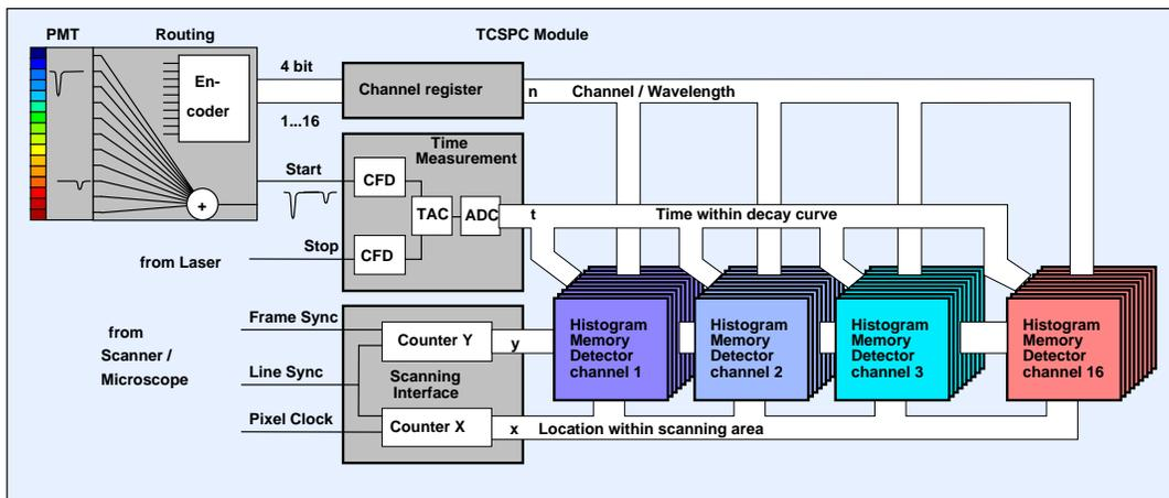
Fig. 7: Combination of multi-dimensional TCSPC with scanning
