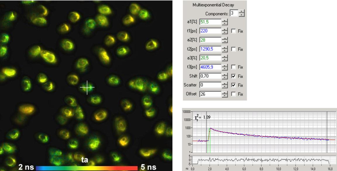
Fig. 10: Lifetime image built up in the time-tag mode. Amplitude-weighted lifetime of triple-exponential decay. Spores of amanita citrina, 512x512 pixels, 256 time channels, Becker & Hickl DCS-120 scanner and SPC-150 TCSPC module
