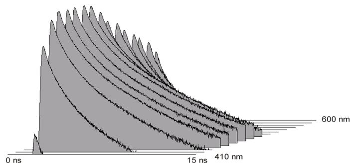
Fig. 3: Fluorescence of human skin, measured by multi-wavelength TCSPC. Excitation wavelength 405 nm, excitation power 60  $\mu$ W, acquisition time 5 s.
