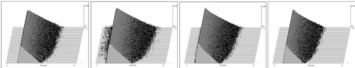
Fig. 6: Photochemical quenching of chlorophyll in a leaf. Fluorescence decay curves in different wavelength channels versus time of exposure. Triggered sequential recording, 50  $\mu$ s per curve, 20,000 on-off cycles accumulated. The sequence starts from the front.
