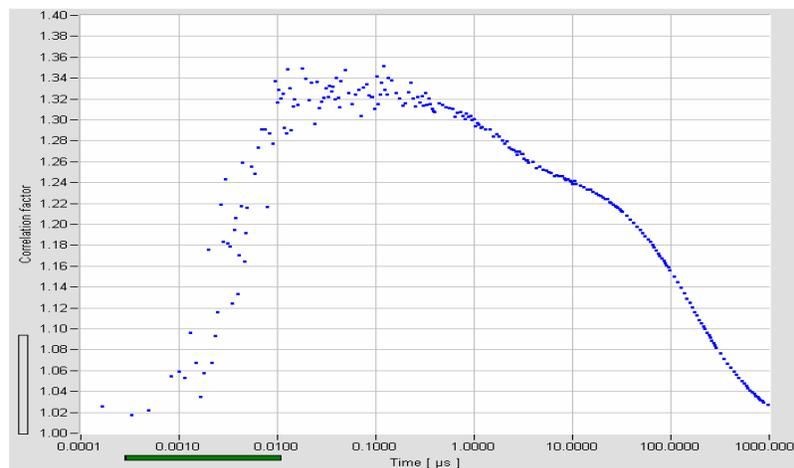
Fig. 11: Fluorescence correlation of a Rhodamin 110 solution over a range from 100 ps to 1 ms. Becker & Hickl DPC-230 TCSPC / Correlator board.
