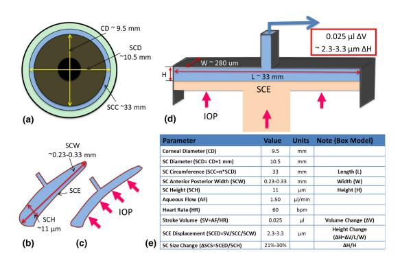
**Fig. 3** SC Deformation Model. (a) Schematic diagram of the front view of the eye. (b) Schematic diagram of the SC cross-section and (c) outward displacement of the SCE into the SC induced by an increase of IOP transient. (d) Schematic diagram of the rectangular box model that approximates the change in the SC volume. (e) Table summarizing the parameters and equations used in the theoretical estimation of the SCE movement.
