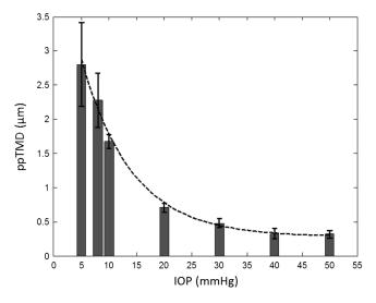
**Fig. 9** Mean and standard deviation of the ppTMD as a function of the mean IOP. The data was fit to an exponential curve.
