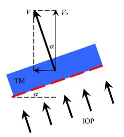
Fig. 2 Schematic diagram of Doppler angle correction.
