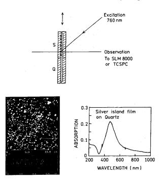
Fig. 1 Sample geometry (top), atomic force microscopy (AFM) image (bottom left) and absorption spectrum (bottom right) SLM8000-spectrofluorimeter.
