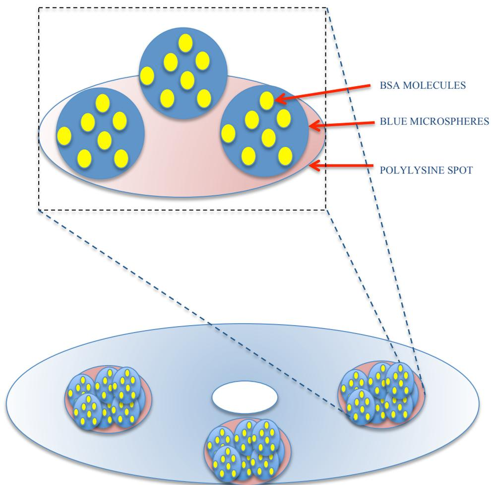
**Fig. 3** Schematics of immobilizing the antibody conjugated polystyrene microparticles to CD surface.
