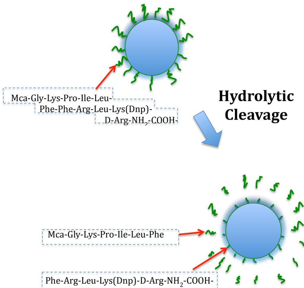
**Fig. 5** Schematic illustration of peptide-conjugated nanoparticles. The peptide sequence is shown. The peptide can be hydrolyzed at the Phe-Phe bond by cathepsin D enzymes and then shows the fluorescence.
