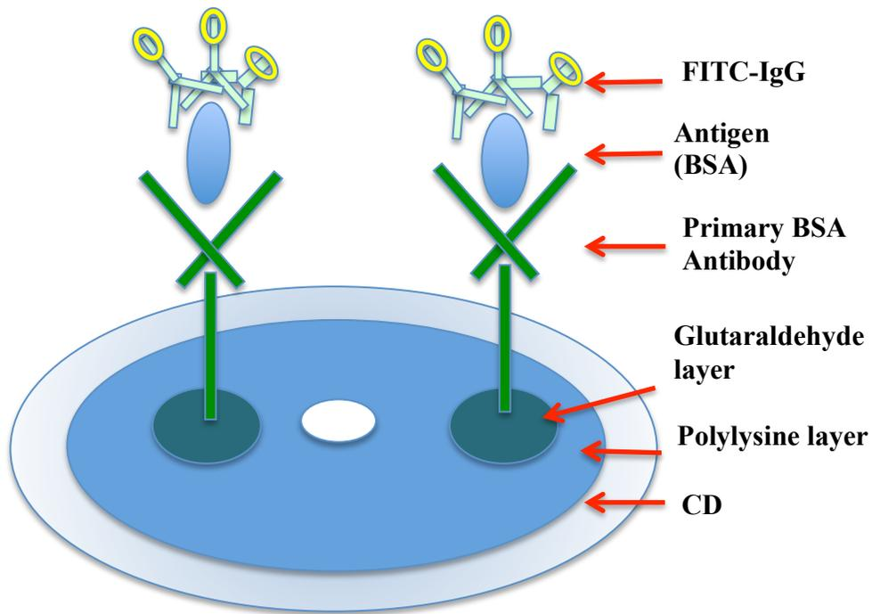
**Fig. 2** Schematics for antibody-antigen conjugation to polycarbonate surface of a compact disk
