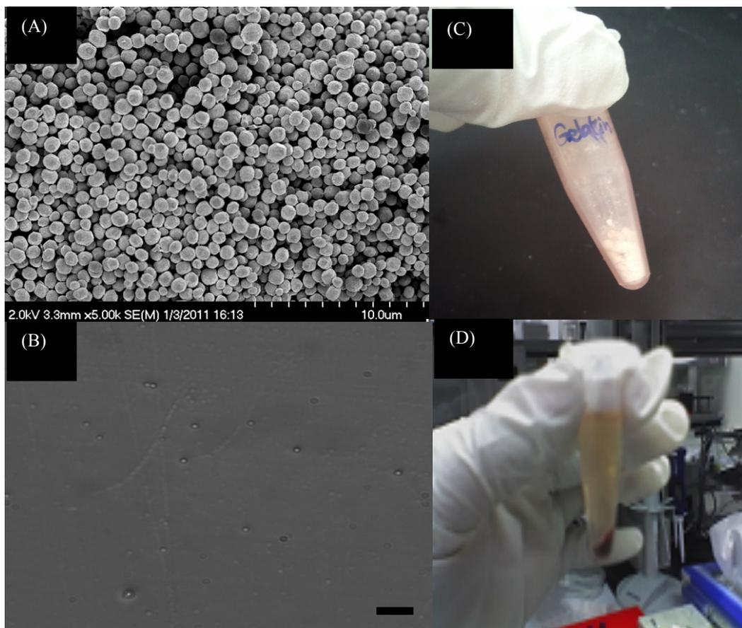
**Fig. 4** (A) Scanning electron microscope images of gelatin submicron particles; (B) Optical image of gelatin particles after swelling in saline solution (200 nm – 5  $\mu$ m); (C) Optical image of dry nanoparticles; (D) Nanoparticles loaded with cancer drug (DOX) after centrifugation. The scale bar represents 10  $\mu$ m.
