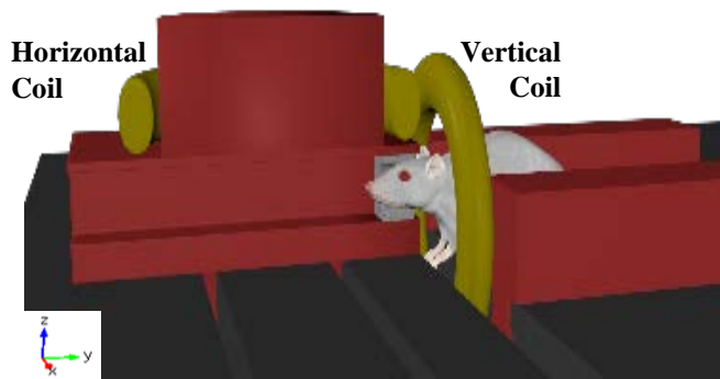
Fig. 2 Side and interior view of coil system with helmet (red) and coils (gold) showing the ability to precisely position mouse relative to coils.
