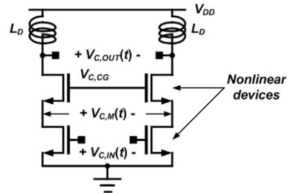
Fig. 1. Typical differential amplifier in the differential mode of operation.
