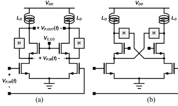
Fig. 2. Proposed harmonic rejection techniques (a) with a simple feedback loop and (b) with a cross-coupled feedback loop.
