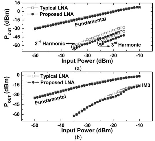
Fig. 6. Measured output power according to the input power: (a) single-tone test and (b) two-tone test.
