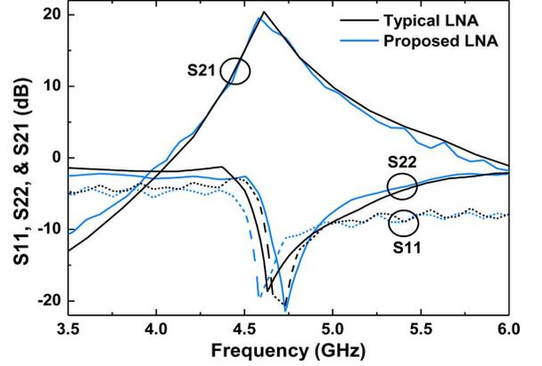
Fig. 5. Measured s-parameters of the proposed LNA.
