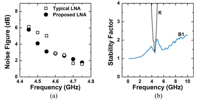
Fig. 7. Measured results: (a) noise figure and (b) stability factor.
