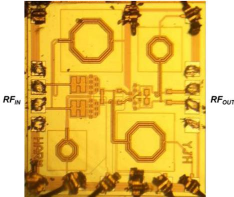
Fig. 4. Photograph of the designed LNA.
