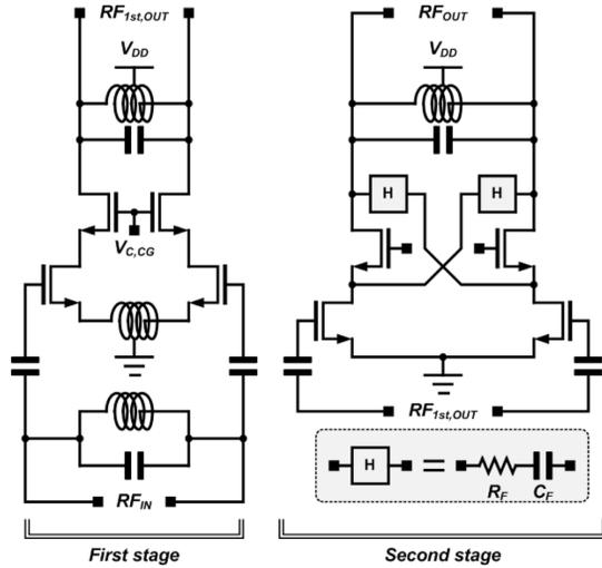
Fig. 3. Simple schematic of the proposed LNA.
