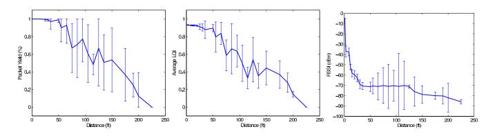
Fig. 5. Packet yield (*left*), link quality indicator (LQI,*center*), and received signal strength (RSSI,*right*) outdoors with the Telos mote and internal antenna. The results are averaged over 10 receivers co-located. From 75-110 feet, a dip in the terrain yields more erratic readings and wider variation in RSSI.
