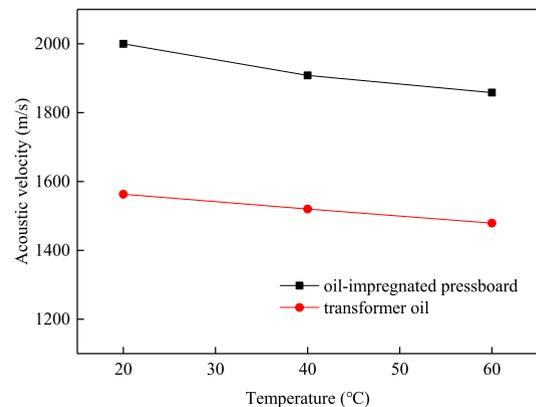
FIGURE 2. Acoustic velocity of transformer oil and oil-impregnated pressboard.
