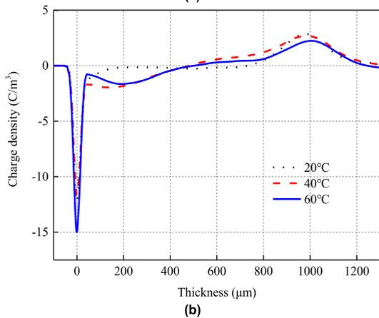
**FIGURE 3.** Space charge distribution of the oil-impregnated pressboard. (a) 10kV. (b) 20kV.
