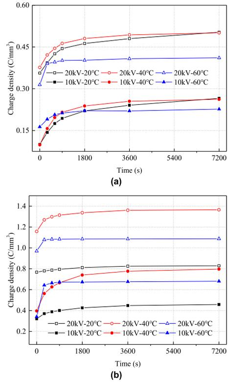
**FIGURE 7. Mean volume density of space charge under different temperature. (a) two layers of oil and pressboard. (b) single layer pressboard.**
