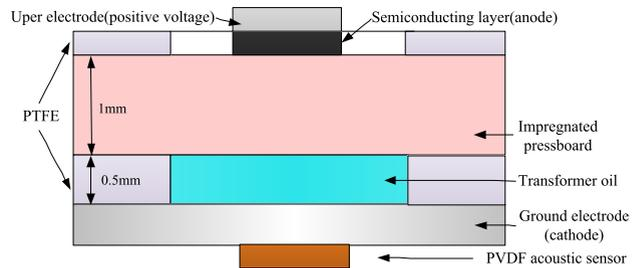
FIGURE 1. Schematic diagram of measuring electrode structure.
