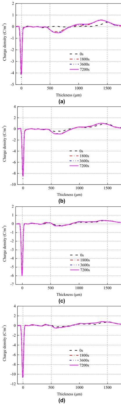
**FIGURE 5.** Space charge distribution of two layers under high temperature. (a) 40°C/10kV. (b) 40°C/20kV. (c) 60°C/10kV. (d) 60°C/20kV.
