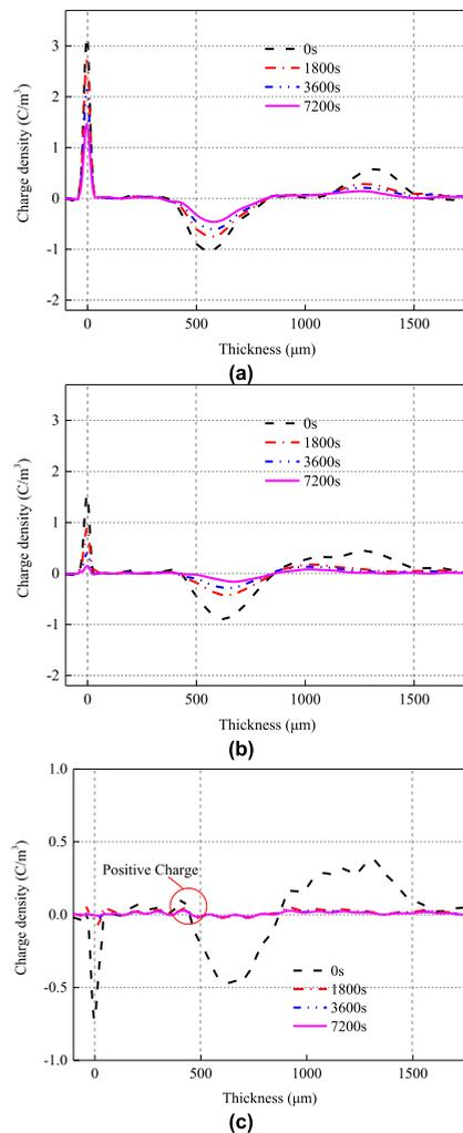
**FIGURE 6.** Space charge distribution during short circuit. (a) 20°C. (b) 40°C. (c) 60°C.
