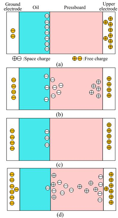
**FIGURE 9.** Schematic diagram of charge distribution. (a) Maxwell-Wagner polarization at 20°C. (b) test results at 20°C. (c) Maxwell-Wagner polarization at 60°C. (d) test results at 60°C.
