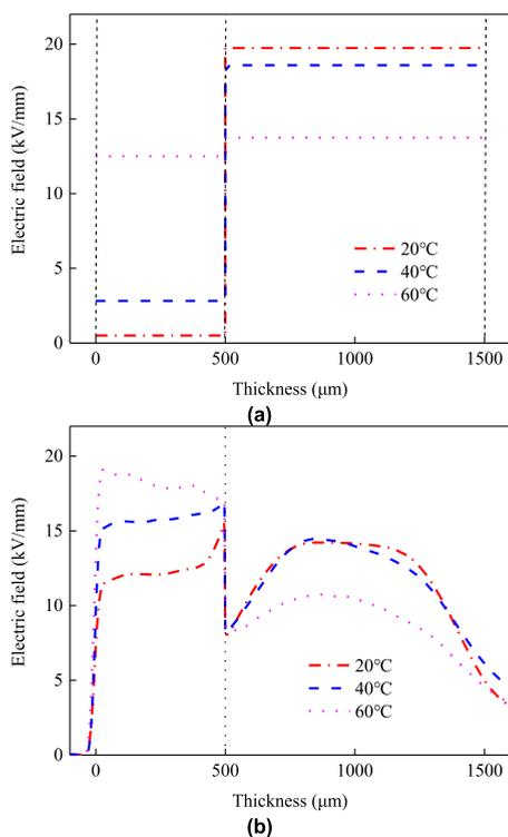
**FIGURE 10.** Electric field distribution in the two layers of oil gap and impregnated pressboard. (a) Maxwell-Wagner polarization under 20kV. (b) calculated by the test results under 20kV.
