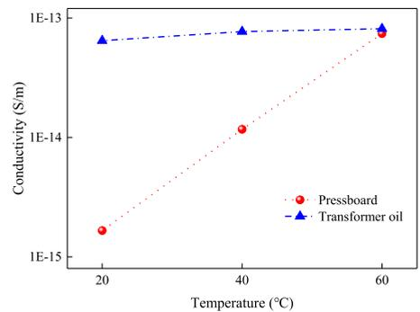
**FIGURE 8. Conductivity of the transformer oil and impregnated pressboard under different temperature.**
