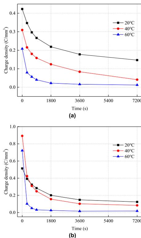
**FIGURE 11.** Mean volume density of space charge during short circuit test. (a) two layers. (b) single layer.
