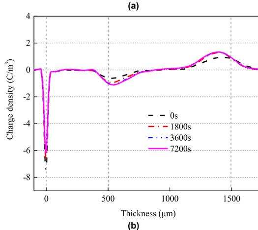
**FIGURE 4.** Space charge distribution in two layers of oil gap and impregnated pressboard at 20°C. (a) 10kV. (b) 20kV.
