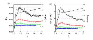
FIG. 3. Normalized real part  $\varepsilon_n'$  (a) and  $\tan \delta$  (b) as a function of  $\lambda$  measured at 7Hz for different strain rates :  $2.5 \times 10^{-3} s^{-1}$  (black triangles),  $2.5 \times 10^{-4} s^{-1}$  (red circles),  $2.5 \times 10^{-5} s^{-1}$  (green squares) and  $2.5 \times 10^{-6} s^{-1}$  (blue diamonds).
