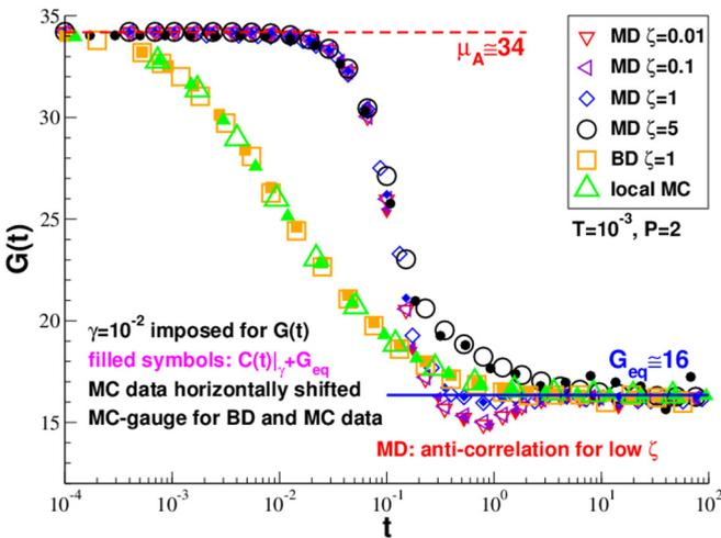
FIG. 4. (Color online) Stress relaxation modulus  $G(t)$  (open symbols) and rescaled autocorrelation function  $C(t)|_\gamma + G_{\text{eq}}$  (filled symbols) for MD simulations for several friction constants  $\zeta$ , BD simulations with  $\zeta = 1$ , and local MC moves. Shifting horizontally the MC data by a factor of  $1/8000$  allows us to bring them to a collapse onto the BD data.
