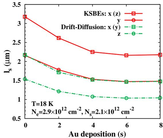
FIG. 4: (Color online) Deposition time dependence of spin diffusion length with the injected spins polarized along the  $x$ -,  $y$ - and  $z$ -axis, respectively. The results from the KSBEs (solid curves) and the two-component drift-diffusion model (chain curves) are both plotted for comparison.
