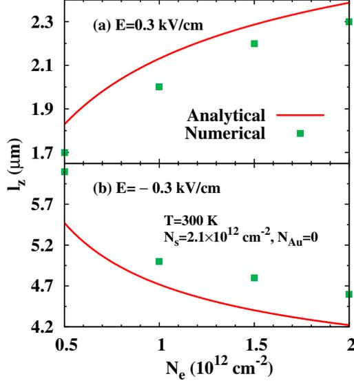
FIG. 7: (Color online) Electron density dependence of spin transport length  $l_z$  under electric fields with opposite directions: (a)  $E = 0.3 \text{ kV/cm}$  and (b)  $E = -0.3 \text{ kV/cm}$ . The squares are from the numerical calculation while the curves are from Eq. (21).  $T = 300 \text{ K}$ ,  $N_s = 2.1 \times 10^{12} \text{ cm}^{-2}$  and  $N_{\text{Au}} = 0$ .
