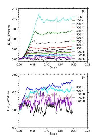
FIG. 3: (a) Potential energy difference (PED) as a function of strain at fixed shear velocity  $v_s = 10^{-3}$  Å/ps for temperatures (from top to bottom) 10 K, 100 K, 200 K, 300 K, 400 K, 500 K, 600 K, 700 K, 800 K, 900 K, 1000 K, 1100 K and 1200 K. For clarity, the high-temperature curves (800-1200 K) are reproduced in (b) on a finer scale.
