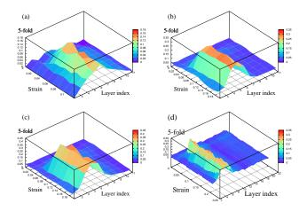
FIG. 6: Fraction of 5-fold coordinated atoms at 300 K as a function of strain and layer index; (a), (b) and (c) correspond to shear velocities (a)  $10^{-5}$  Å/ps, (b)  $10^{-3}$  Å/ps, and (c)  $10^{-1}$  Å/ps, at 300 K. The configurations are divided into 12 layers along the *y*-direction; layers 1 and 12 are not shown as they correspond to the frozen walls. The figure (d) correspond to a system of 16000 particles and a shear velocity of 5 ×  $10^{-4}$  Å/ps. The number of layers is 22.
