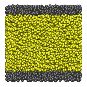
FIG. 1: Snapshot of a typical configuration of the 8000particle *a*-Si-model. Mobile particles are positioned between two parallel walls, each containing 1000 atoms, used for applying the shear deformations (see text for more details).
