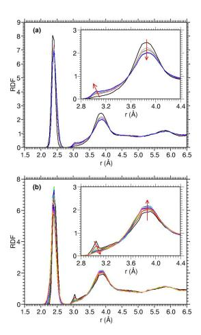
FIG. 4: Radial distribution function (a) as a function of shear velocity at 300 K, and (b) as a function of temperature at  $v_s = 10^{-3}$  Å/ps. The arrows indicate the direction of increasing shear velocity or temperature (see text).
