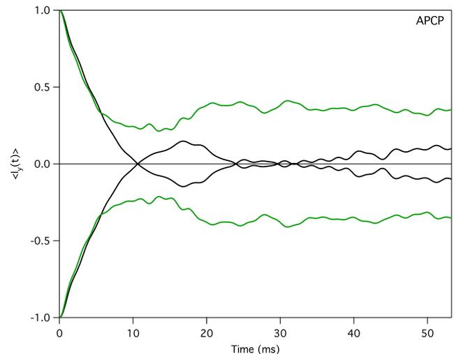
FIG. 27: (Color online) Calculations for APCP with  $N = 4$ ,  $\Omega_z$  drawn from a 290 Hz wide Gaussian,  $1 \times B_{jk}$  of  $^{29}\text{Si}$  in silicon,  $H_1 = 1.5$  MHz,  $2\tau = 2 \mu\text{s}$ , and 100 DR average. Even for  $H_1/\text{FWHM} = 5000$ , the delta-function pulse approximation (black) misses important physics from the exact calculation (green).
