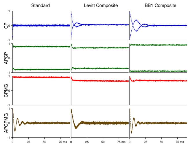
FIG. 14: (Color online) Pulse sequences CP, APCP, CPMG, and APCPMG using standard  $\pi$  pulses (left column), Levitt composite  $\pi$  pulses (middle column), and BB1 composite  $\pi$  pulses (right column).  $H_1 = 35.7$  kHz,  $2\tau = 72$   $\mu$ s,  $T = 300$  K,  $B^{\text{ext}} = 11.74$  Tesla.
