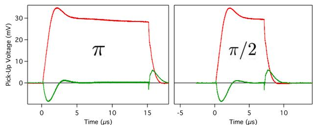
FIG. 12: (Color online) Measured pulse shapes in-phase (red) and out-of-phase (green) for a typical  $\pi$  pulse (left) and  $\pi/2$  pulse (right) at radio frequency 101.5 MHz with pulse strength  $H_1 = 33.3$  kHz. Transients are a larger fraction of short duration pulses like  $\pi/2$ . Data taken at room temperature in a 12 Tesla field. The real  $\pi$  pulse is approximated as three pure rotations  $4_X 180.1_Y 3_X$ .
