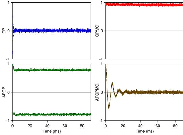
FIG. 6: (Color online) Four pulse sequences with  $\pi$  pulses of different phases applied to  $^{29}\text{Si}$  in Si:Sb ( $2.75 \times 10^{17} \text{ Sb/cm}^3$ ). (Top Left) CP, (Top Right) CPMG, (Bottom Left) APCP, (Bottom Right) APCPMG. All are expected to yield identical decay curves.  $2\tau = 72 \mu\text{s}$ ,  $T = 300 \text{ K}$ , and  $B^{\text{ext}} = 11.74 \text{ Tesla}$ .
