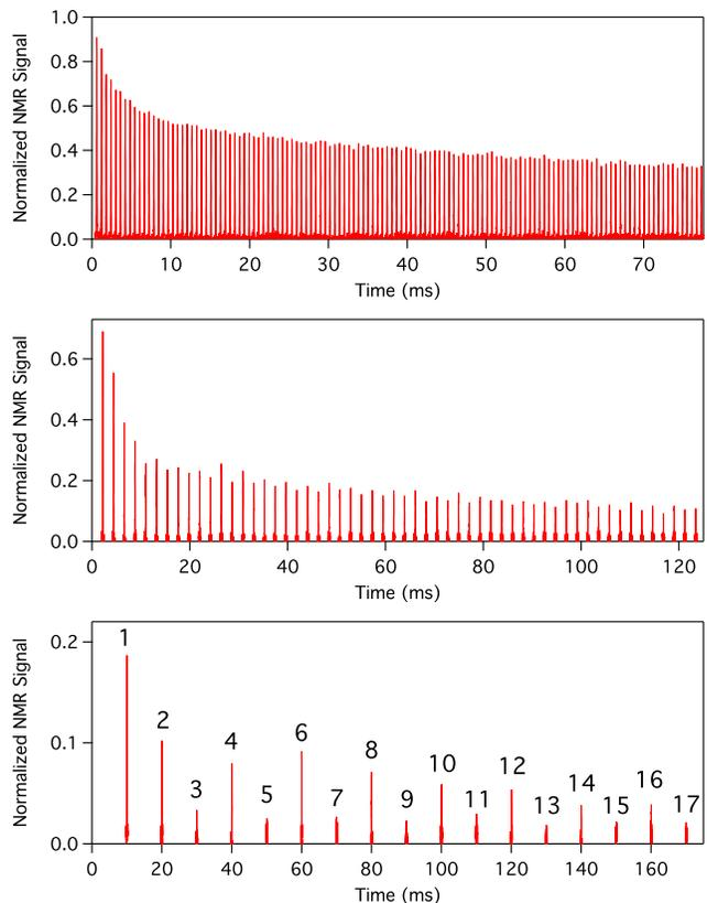
FIG. 4: (Color online) CPMG echo trains of  $^{29}\text{Si}$  in Si:P ( $3.94 \times 10^{19}$  P/cm<sup>3</sup>) with three time delays between  $\pi$  pulses. (Top)  $2\tau = 592 \mu\text{s}$ . (Middle)  $2\tau = 2.192$  ms. (Bottom)  $2\tau = 9.92$  ms. For comparison,  $T_2 = 5.6$  ms in silicon as measured by the Hahn echoes and as predicted by the delta-function pulse approximation. Data taken at room temperature in a 12 Tesla field.
