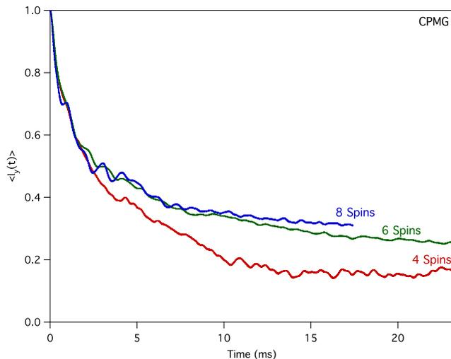
FIG. 22: (Color online) Exact calculations of the CPMG pulse sequence show that the tail height of the measurable coherence increases with system size (even  $N$  are compared to avoid artifacts<sup>93</sup>). Parameters:  $\Omega_z = 0$ ,  $H_1 = 40$  kHz,  $2\tau = 2 \mu\text{s}$ ,  $25 \times B_{jk}$  of  $^{29}\text{Si}$  in silicon with a dipolar linewidth of 2.2 kHz, 400 DR average (100 DR average for  $N=8$ ).
