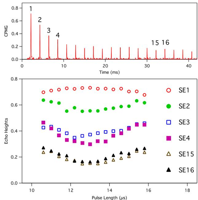
FIG. 9: (Color online) Finding the minimum tail height for CPMG. (Top) CPMG data of  $^{29}\text{Si}$  in Si:P ( $3.94 \times 10^{19}$  P/cm $^3$ ) with  $2\tau = 2.192$  ms. (Bottom) Numbered spin echoes (SE $n$ ) are plotted versus  $\pi$  pulse duration. SE15 and SE16 are expected to have zero amplitude. The nutation calibrated  $\pi$  pulse has duration  $12.2 \mu\text{s}$ . Data taken at room temperature in a 12 Tesla field.
