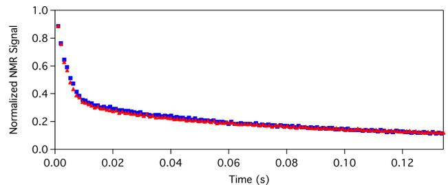
FIG. 16: (Color online) Temperature effects on CPMG tail height. CPMG echo peaks at room temperature (red) and 4 Kelvin (blue) in Si:P ( $3.94 \times 10^{19}$  P/cm $^3$ ) diluted in paraffin wax.  $2\tau = 2.192$  ms,  $B^{\text{ext}} = 12$  Tesla.
