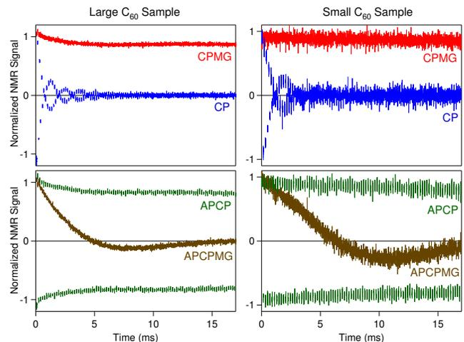
FIG. 11: (Color online) Pulse phase sensitivity and rf homogeneity tests in an insulating sample. CP, CPMG, APCP, and APCPMG data of  $^{13}\text{C}$  in  $\text{C}_{60}$  for a large sample volume (left column) and a small sample volume (right column). All are expected to agree in the delta-function pulse limit.  $H_1 = 45.5$  kHz,  $^{13}\text{C}$  NMR linewidth = 290 Hz,  $2\tau = 180$   $\mu\text{s}$ ,  $T = 300$  K,  $B^{\text{ext}} = 12$  Tesla.
