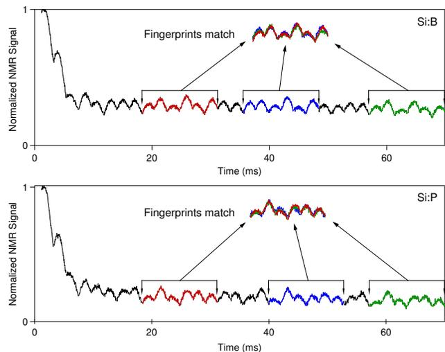
FIG. 5: (Color online) Repeated fingerprint patterns in the CPMG echo train with  $2\tau = 2.192$  ms. Two different samples are shown: (top) Si:B ( $1.43 \times 10^{16}$  B/cm<sup>3</sup>), and (bottom) Si:P ( $3 \times 10^{13}$  P/cm<sup>3</sup>). Data taken at room temperature in a 7 Tesla field.
