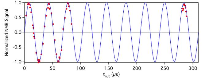
FIG. 7: (Color online) Nutation curve data (dots) of  $^{29}\text{Si}$  in Si:Sb ( $2.75 \times 10^{17} \text{ Sb/cm}^3$ ) agree with a non-decaying sine curve over 8.25 cycles.  $H_1 = 8.33 \text{ kHz}$ ,  $T = 300 \text{ K}$ , and  $B^{\text{ext}} = 12 \text{ Tesla}$ .
