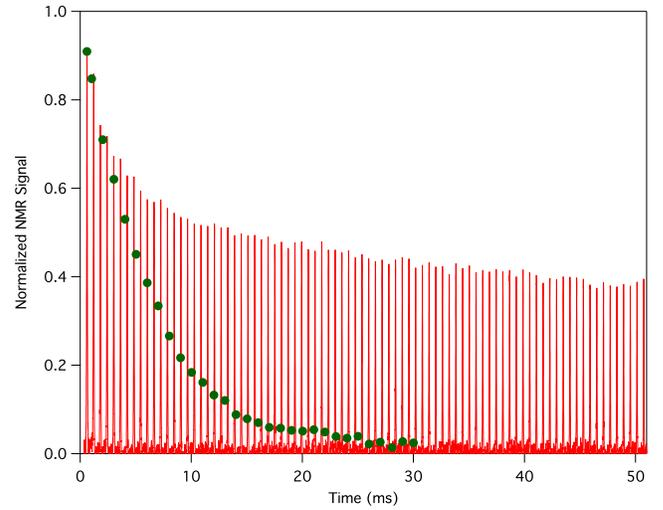
FIG. 1: (Color online) Two NMR experiments to measure  $T_2$  of  $^{29}\text{Si}$  in a crushed powder of Silicon doped with Phosphorous ( $3.94 \times 10^{19} \text{ P/cm}^3$ ). Hahn echo peaks (dots) are generated with a single  $\pi$  pulse. The CPMG echo train (lines) is generated with multiple  $\pi$  pulses spaced with delay  $2\tau = 592 \mu\text{s}$ . Normalization is set by the initial magnetization after the  $90_X$  pulse. Data taken at room temperature in a 12 Tesla field.
