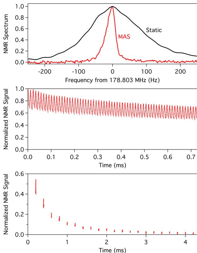
FIG. 18: (Color online) Magic Angle Spinning in Si:Sb ( $10^{17}$  Sb/cm $^3$ ). (Top) NMR spectrum of a static powdered sample with FWHM = 175Hz (black) and the MAS spectrum spun at 3 kHz with FWHM = 31 Hz (red). (Middle) CPMG echo train while spinning.  $2\tau = 11.25$  ms. Long tail is expected since dipolar coupling is reduced. (Bottom) CPMG echo train while spinning.  $2\tau = 0.2$  s. No pronounced even-odd effect, in contrast to Fig. 4(bottom) and Fig. 17(bottom).
