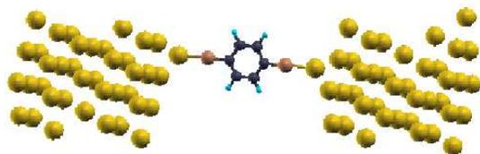
FIG. 13: (Color on line) BDT molecule attached to adatoms at both of the Au (111) surfaces. Color code: Au=yellow (or light gray), C=black, S=dark yellow (or gray), H=blue (or dark gray).
