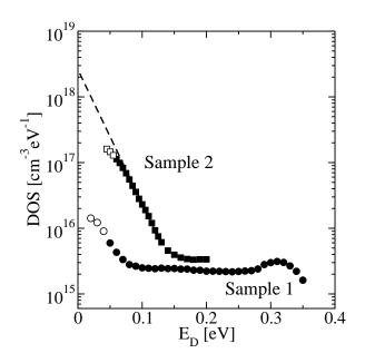
FIG. 6: The density of states toward midgap is in the range of  $10^{15}$  cm<sup>-3</sup>eV<sup>-1</sup>. Close to the band edge, the DOS increases in a way reminiscent of band tail states (sample 2). Within 2–3kT to the mobility edge, the analysis starts to fail, causing an unphysical roll-over of the DOS (open symbols).
