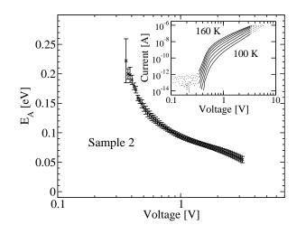
FIG. 5: Activation energy  $E_{\rm A}(V)$  for sample 2. Inset: *I*-*V* curves for sample 2. Below 0.34 V, where the current is contact-limited, as well as above 3.3 V, close to the rollover to a  $I \propto V^2$  behavior, the current is not thermally activated. Thus meaningful activation energies can be extracted only in this intermediate range. Consequently, only data represented by solid lines was used for the extraction of  $E_{\rm A}(V)$  and the  ${\rm DOS}(E)$ .
