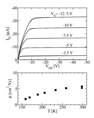
FIG. 3: Single-crystal field-effect-transistors: The upper panel shows the output characteristic of a flip-crystal FET measured at room temperature. (Dimensions:  $W=770\mu$ m,  $L=100 \mu$ m,  $d_{\rm SiO_2}=300$  nm.) Lower panel: Mobility  $\mu$  for a flip crystal FET as a function of temperature, indicating a slight decrease from 6 cm<sup>2</sup>/Vs at room temperature to 2 cm<sup>2</sup>/Vs at 160 K.
