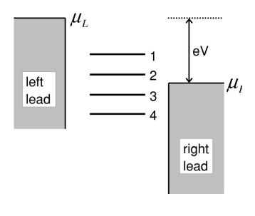
FIG. 1. Schematic setup for electrical transport through a multilevel mesoscopic system.
