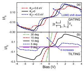
FIG. 4. Current-voltage characteristic and effects of gating and tilting with respect to the Au(111) electrode surface on current through the BDT molecule on the top site: (a) effect of the gating, onsite energies are shifted by the amount  $\Phi_g$  indicated on the figure, (b) effect of increasing tilt angle  $\theta$ . Current is in units of  $I_0=77.5\mu A$ . Inset: schematic of the gate geometry, 2t=1 nm, L=4-5 nm (nominal oxide thickness was 30nm),  $V_g$  is the gate voltage.
