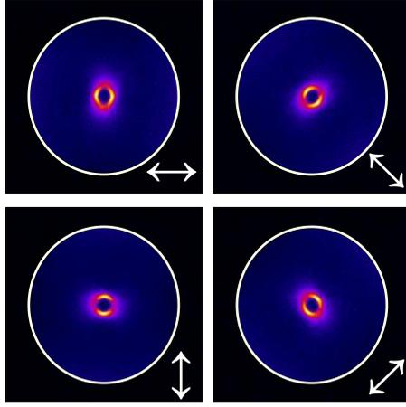
FIG. 3. Images of the back focal plane at 1050 nm for the  $m=3$  structure already studied in Fig. 1 (the same color code has been used). Here, a linear polarizer is inserted in front of the InGaAs camera. The orientation of the polarization axis is indicated with the double arrows on each panel.
