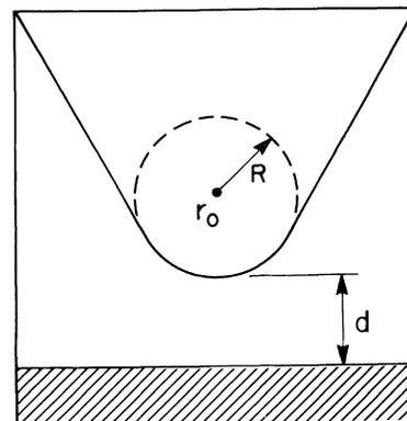
FIG. 1. Schematic picture of tunneling geometry. Probe tip has arbitrary shape but is assumed locally spherical with radius of curvature  $R$ , where it approaches nearest the surface (shaded). Distance of nearest approach is  $d$ . Center of curvature of tip is labeled  $\vec{r}_0$ .
