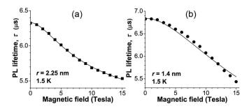
FIG. 4: Magnetic fields reduce  $\tau$  at low T (1.5 K), for both (a) large and (b) small PbSe NCs. In large NCs, where Zeeman energies are large but  $\Delta$  is small (see text),  $\tau$  begins to saturate above 10 T. Lines show fits to the model of [27].
