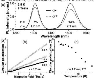
FIG. 5: (a) Circularly-polarized infrared PL emission from PbSe NCs at B=7 T and T=2.5 K. (b) PL polarization versus B. (c) PL polarization vs. T at B=7 T.
