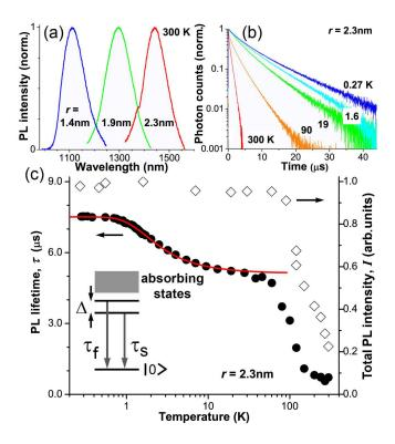
FIG. 1: (a) PL spectra from PbSe NC ensembles of different size. (b) PL decays. The lifetime  $\tau$  increases as temperature T decreases. (c) Left axis:  $\tau$  versus T from 270 mK to 300 K. Line is a fit of the low-T data to a two-level model (see inset). Right axis: The integrated PL emission, I. Note both  $\tau$  and I increase ~fivefold upon cooling to 50 K in these NCs, indicating freeze-out of competing non-radiative recombination channels. I remains unchanged below 50 K.
