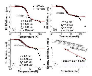
FIG. 2: (a-c)  $\tau$  vs. T for three PbSe NC sizes at B=0 T (black points). Lines are fits to a two-level model (see text). Open symbols show  $\tau(T)$  at B=15 T. High fields reduce  $\tau$  to its value at ~10 K. (d) The energy splitting  $\Delta$  between these two lowest exciton levels versus NC radius.
