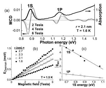
FIG. 3: (a) Optical absorption (right axis) and corresponding magnetic circular dichroism (MCD; left axis) from r=2.1 nm PbSe NCs. (b) Zeeman splitting of the 1S absorption feature, for different NCs. (c) The effective exciton g-factor  $|g_{ex}|$  versus 1S band-gap energy.
