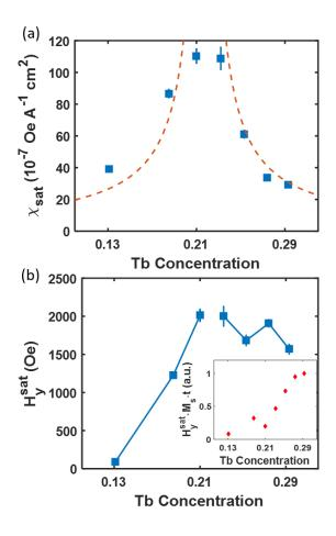
Fig. 4 (a) Saturation efficiency and (b) in-plane saturation field for different  $Co_{1-x}Tb_x$  films. Both the saturation efficiency and in-plane saturation field are largest near the magnetic moment compensation point. The dashed line in (a) shows the trend calculated from  $\chi_{sat} \sim 1/M_s t$ . Inset of (b) plots the product of the in-plane saturation field and magnetic moment  $M_s t$ , indicating an increase in DMI energy density D with increasing Tb concentration.
