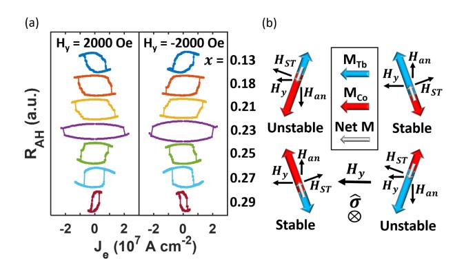
Fig. 2 (a) Current induced SOT switching of  $Co_{1-x}Tb_x$  for in-plane fields of  $\pm$  2000 Oe. The current density inside Ta is calculated based on the conductivity of Ta thin films. (b) Schematic of effective fields in a ferrimagnetic system. Fields acting on the moment consist of the in-plane field H<sub>y</sub>, the anisotropy field H<sub>an</sub>, and the SOT field H<sub>ST</sub>.
