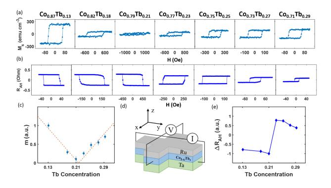
Fig. 1 (a) Out of plane magnetization curves of  $Co_{1-x}Tb_x$  films. (b)  $R_{AH}$  as a function of perpendicular magnetic field. (c) Magnetic moments of  $Co_{1-x}Tb_x$  alloys as a function of Tb concentration. (d) Schematic of the device geometry for  $R_{AH}$  measurement. (e)  $R_{AH}$  as a function of Tb concentration.
