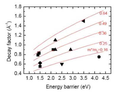
Fig. 3. Left: Tunnel decay factor – energy barrier plot for several molecular tunnel junctions:
