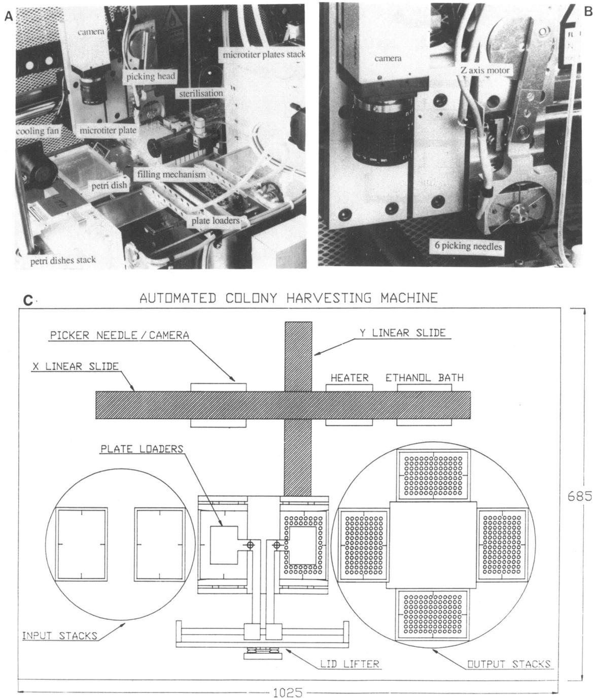
**Figure 1.** Plan and details of the automated colony picker. A) view of the main working components of the system showing their relative positions. B) close up view of the camera and z axis with 6 way picker needles. C) drawing of a plan view of the machine giving overall dimensions and layout.
