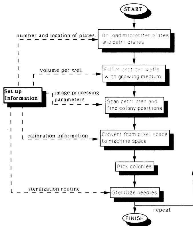
**Figure 2.** Flow diagram of machine operations. Solid lines show the logical flow of operations and dotted lines show information flow from the start up parameters.
